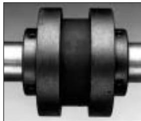
**Step 5.** Slide loose flange on the shaft until the sleeve has seated completely in teeth of both flanges. Refer to "Y" dimension although not a critical dimension. Secure the flange to shaft and torque set screws and cap screws to correct torque values.
